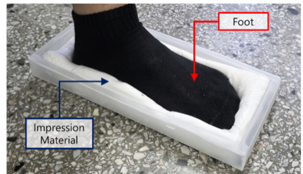
Fig. 2 Photograph showing the subject capturing the plantar shape using the impression-based acquisition kit
