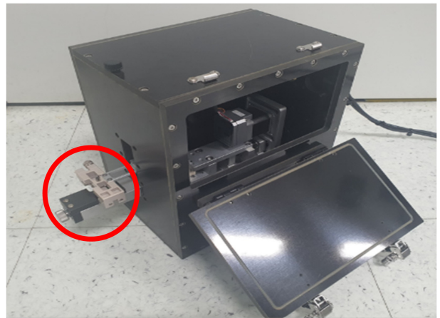
Fig. 3 Manufactured fretting corrosion test jig box
