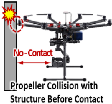
Fig. 2 Example of propeller collision with structure before contact in the SAM system
