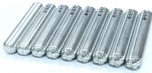
Fig. 9 Visual appearance of forged workpieces with increasing number of passes
