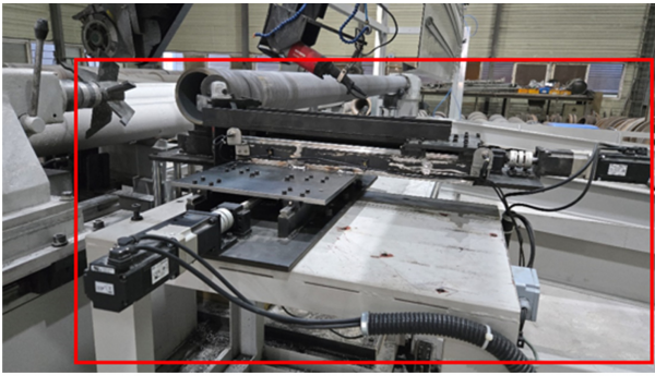
(a) Fabricated cylindrical chamfering device
