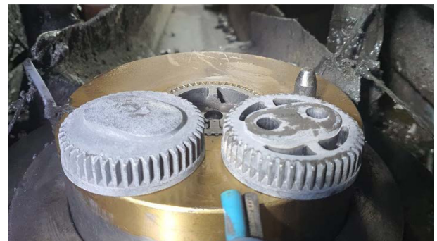
Fig. 16 Final cold forging process of spur gear die for hedge trimmer
