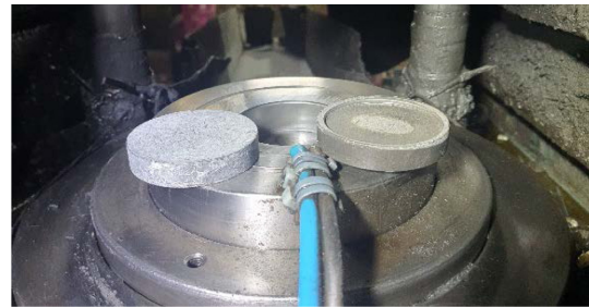
Fig. 14 1st cold forging process of spur gear die for hedge trimmer
