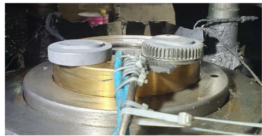
Fig. 15 2nd cold forging process of spur gear mold for hedge trimmer
