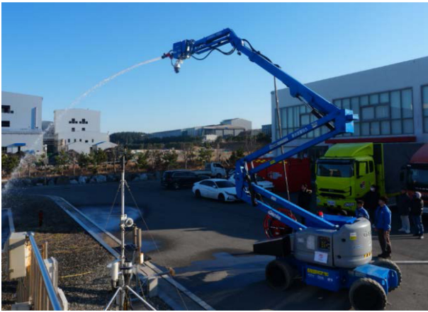
Fig. 13 Water spray test verifying fluid supply stability during lift extension
