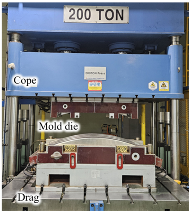
Fig. 2 A set up of PCM process to manufacture leaf spring
