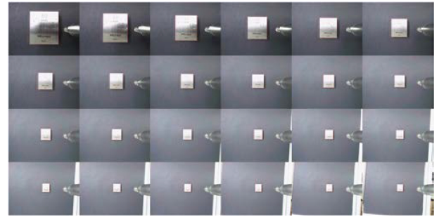
Fig. 9 Calibration image using block gauges by distance
