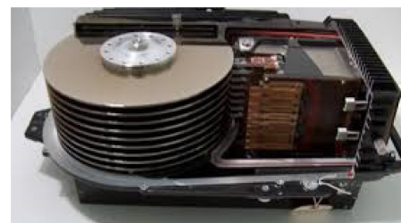
Fig. 2 The last HDD for main-frame computers: IBM 3390 introduced in 1989 - the maximum capacity was up to 22.7 GB
