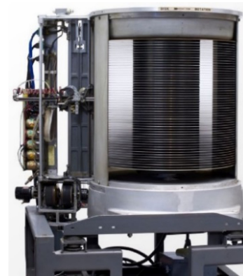
Fig. 1 The first computer hard disk drive introduced in 1956: IBM 350 disk storage unit for IBM 305 RAMAC system
