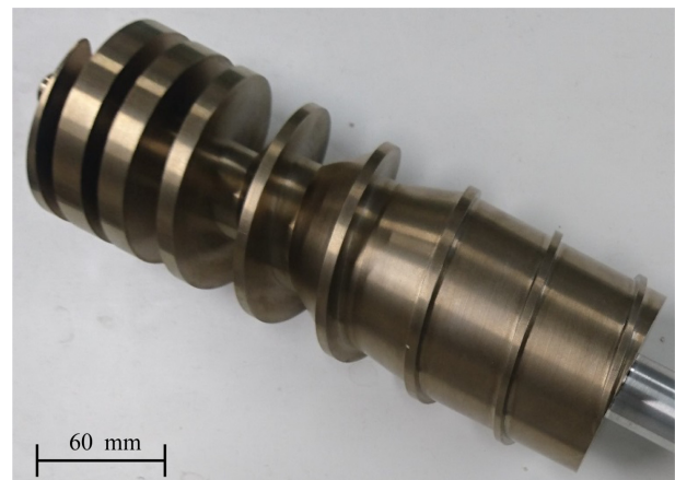
Fig. 2 Example of variable pitch screw (2)
