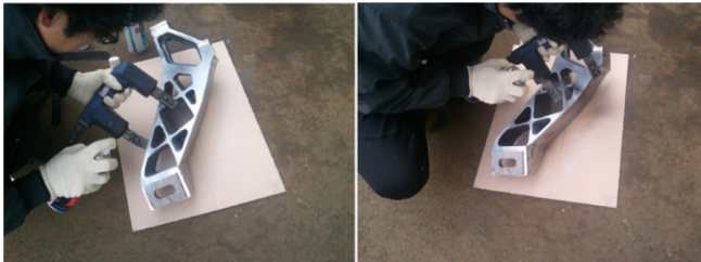
Fig. 10 Perform magnetic particle inspection before test
