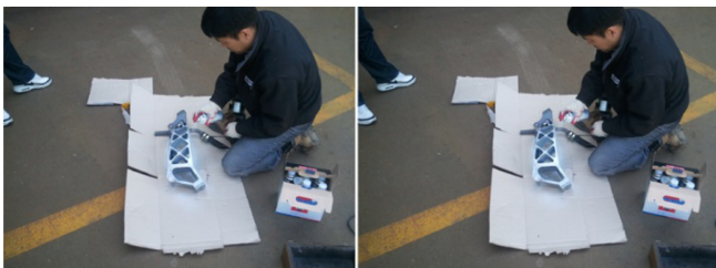
Fig. 11 Perform magnetic particle inspection after test
