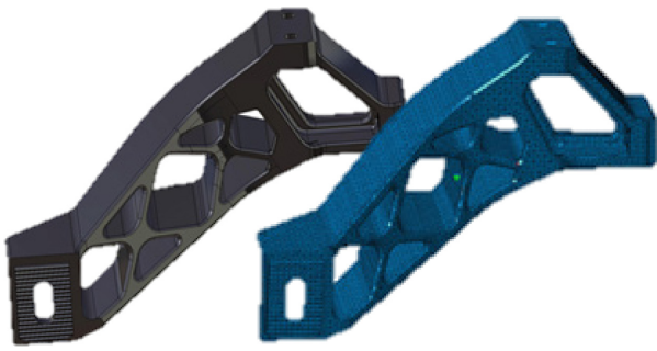
Fig. 4 Sanding device support bracket analysis model
