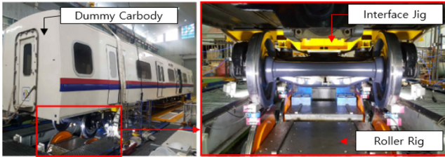
Fig. 10 Test condition for running behavior measurement at laboratory environment
