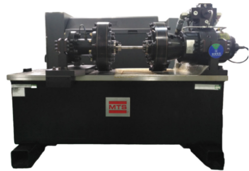
Fig. 8 MTS torsional fatigue testing machine
