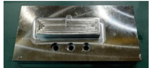
Fig. 12 Finished test piece after post-process machining
