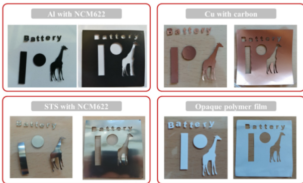
Fig. 5 Laser cutting results of the battery materials with various patterns
