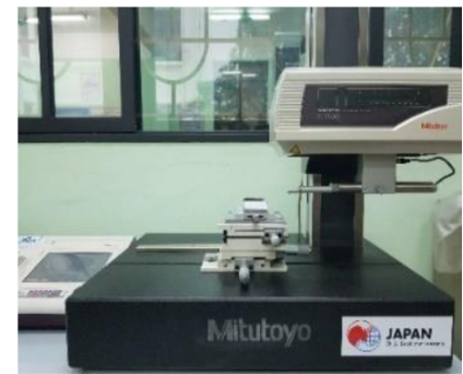
Fig. 2 Mitutoyo Surftest SV-2100 surface roughness tester
