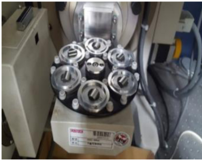
Fig. 3 XRD system for measuring residual stress
