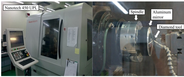
Fig. 2 Nanotech 450 UPL (Left) and SPDT machining of an aluminum mirror (Right)
