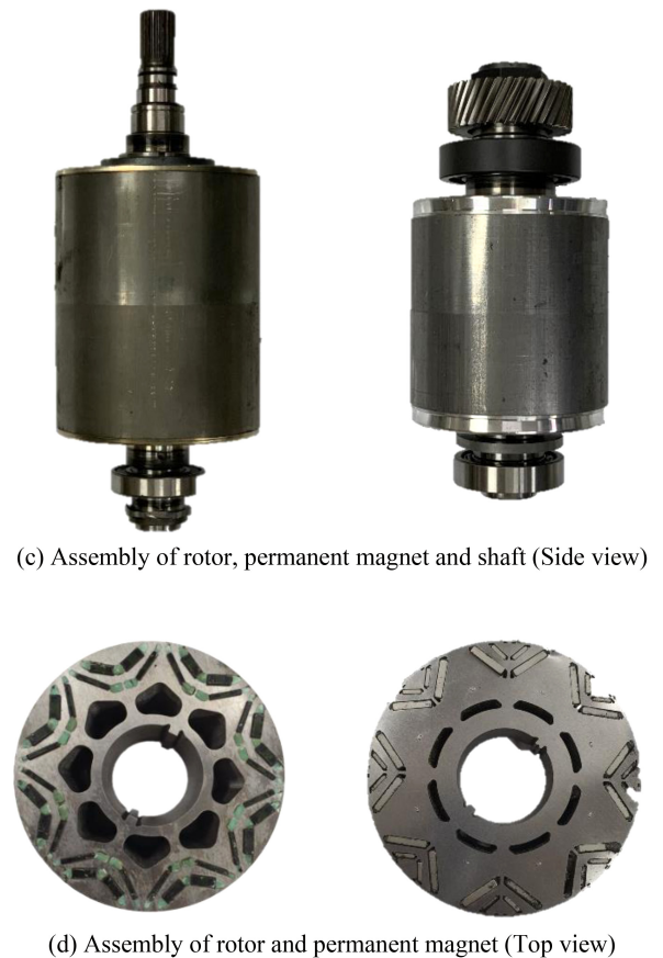
Fig. 2 Actual photograph of direct tear-down stator and rotor parts of electric motor model N (Left) and B (Right)
