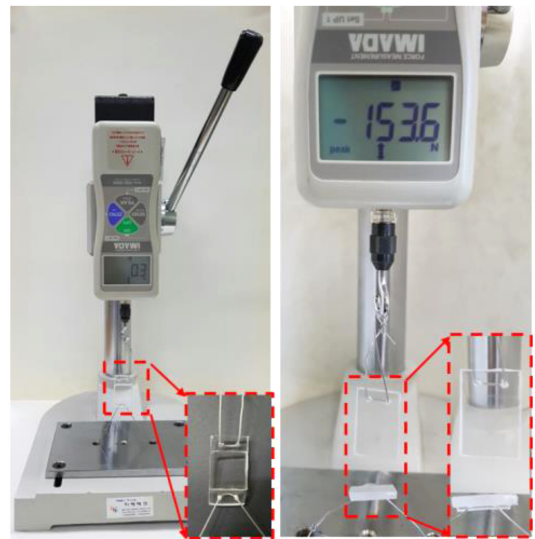
Fig. 5 Bonding strength test using tension and compression tester
