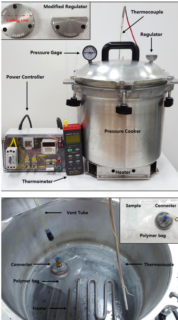
Fig. 3 PMMA thermal bonding system and chamber inside
