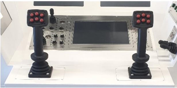
Fig. 12 Joystick interface for micro operation
