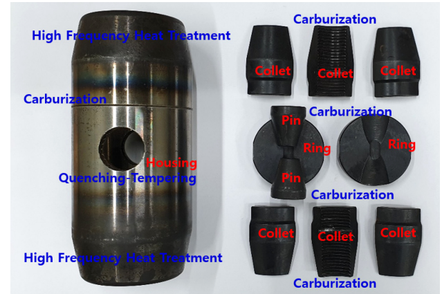
Fig. 1 Coupler configuration diagram
