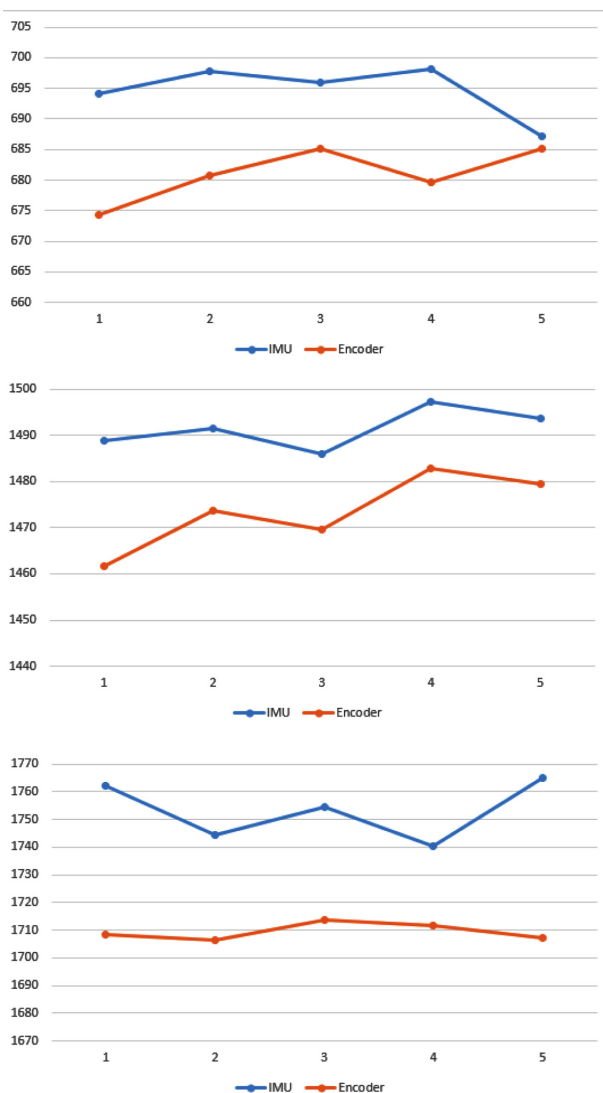
Fig. 9 Comparative measurement result of IMU and encoder
