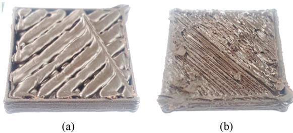
Fig. 9 Geometrical shape of fabricated chocolate with different nozzle diameter (30 × 30 × 5 mm)
