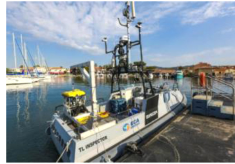
(a) Inspector USV with H300V UUV
