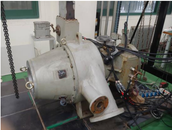
Fig. 6 Prototype compressor for 340 kW chiller. The cooling capacity is 500RT
