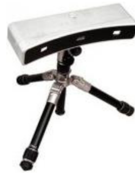
Fig. 5 The 3D scanner used for measuring dimensional accuracy of bone plates
