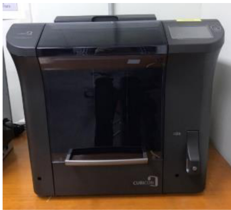
Fig. 4 The FDM 3D printer used for bone plates printing
