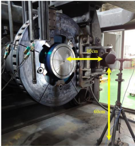
Fig. 7 The squeal noise measuring experiment for the railway brake system in dynamometer
