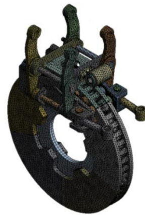
Fig. 10 The finite element model of the brake system with the flexible pad. The total number of elements was 399,642
