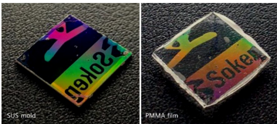
Fig. 6 Photographs of fabricated nanopatterned mold deposited on stainless steel using polymer nanocomposite (Left) and hot-embossed PMMA film (Right)
