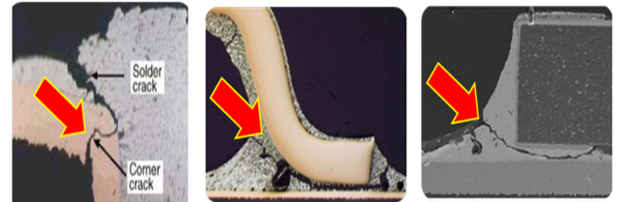
Fig. 2 Main failure mode of electronic control unit
