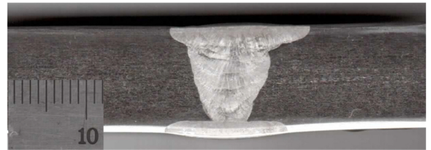
Fig. 1 Inconel 617 alloy welded block
