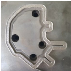
(a) Deposition of M2 material on the base of mold
