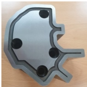
(b) Final 3D printed blanking mold
