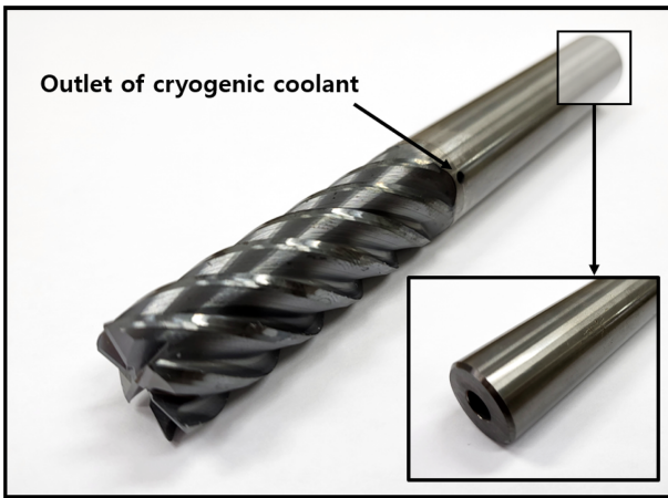
Fig. 2 Cryogenic machining tool including indirect spraying system
