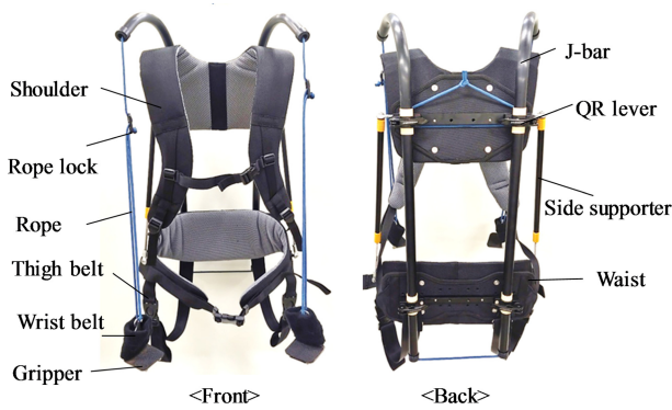
Fig. 1 Elements of the H-Frame
