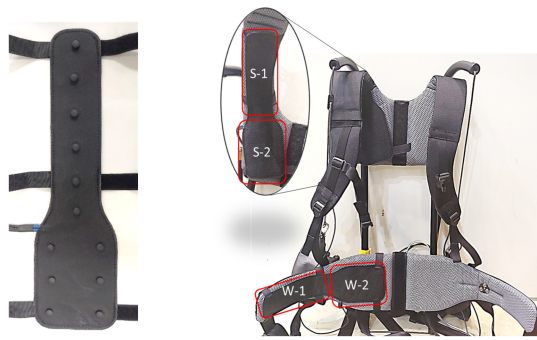
(a) Compression force sensor (b) Location of the sensor
