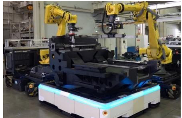
Fig. 7 Cooperation assembly of two robots
