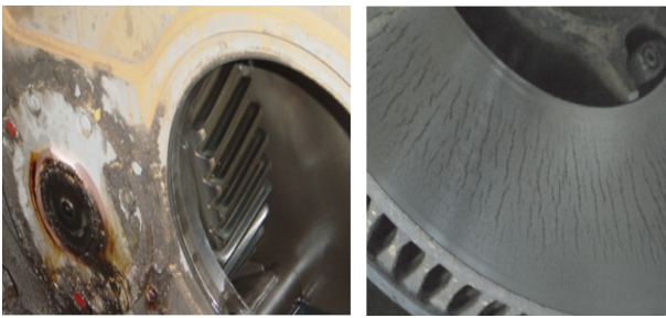
Fig. 1 Failures of driving gear box and brake disc
