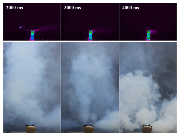
Fig. 7 Visualization of gas emitted during internal short circuit during thermal runaway step of SOC 40% 18650 cell
