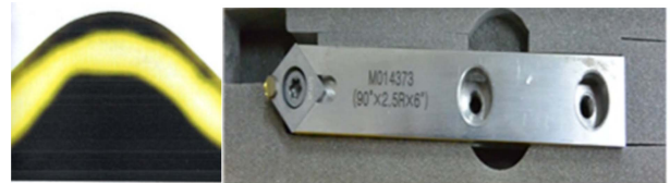
Fig. 15 Diamond tools of fine servo
