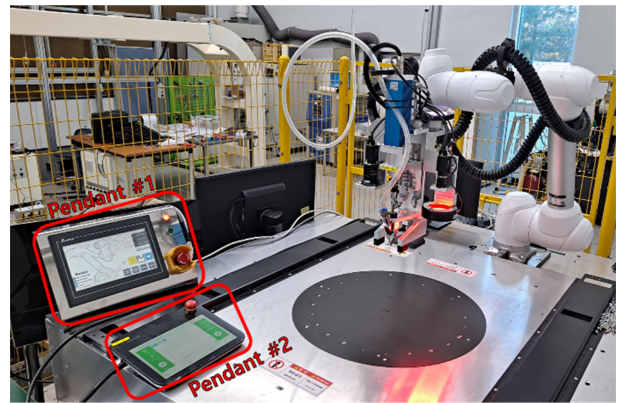
Fig. 4 Overview of screwing automation robot system
