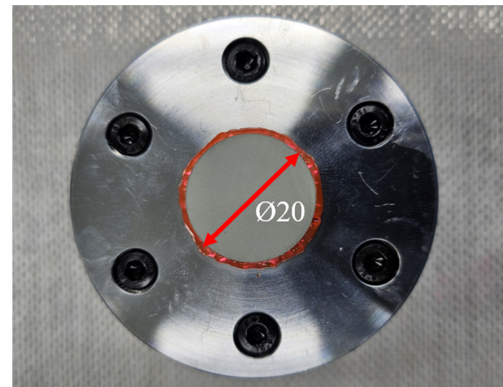
Fig. 1 Germanium (Ge) sample with machining jig
