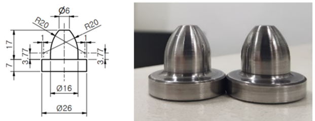
Fig. 3 Dimension and shape of electrode
