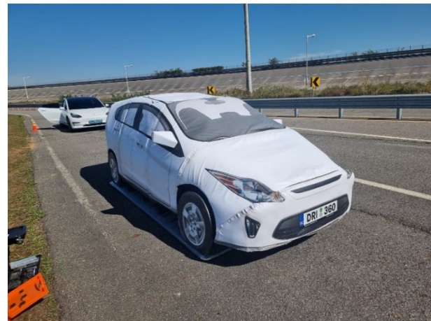
Fig. 2 Guided vehicle target robot with dummy
