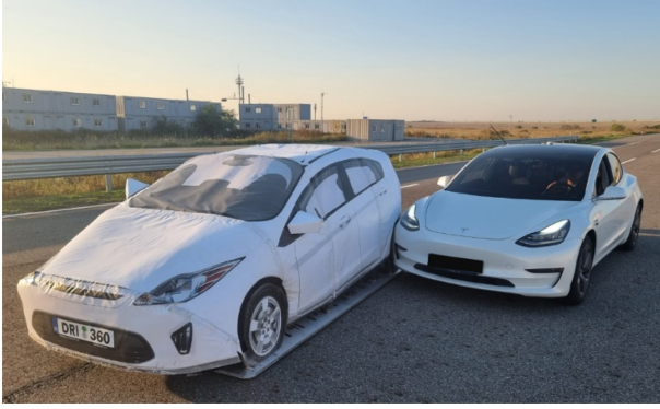
Fig. 4 Guided vehicle target robot test
