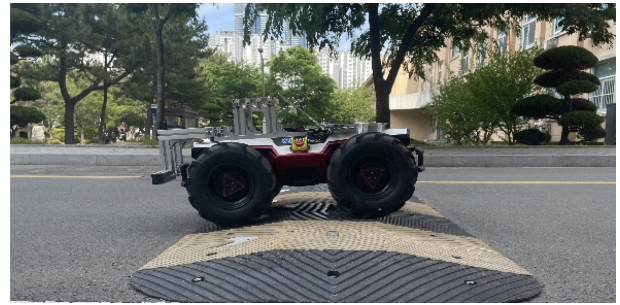
Fig. 11 Bump running experiment
