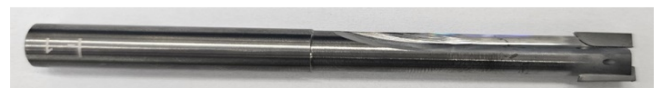
Fig. 9 CAD design and brazing images of PCD tip reamer: (a) 2D CAD of PCD tip reamer and (b) Image of the brazed reamer
