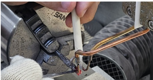
Fig. 4 Image of the improved coil
