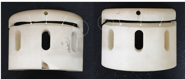
Fig. 20 Location of failure for alumina specimen holder after thermal gradient test
