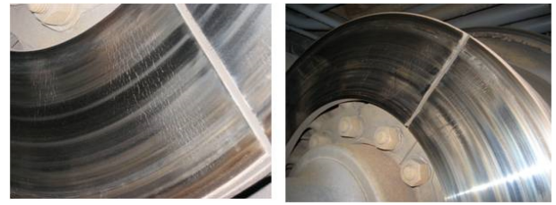
Fig. 1 The brake disc showing the radial distribution of thermal cracks
