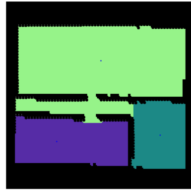
Fig. 9 Morphological segmentation is the result of area division
