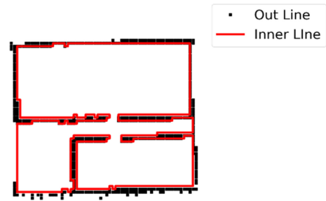
Fig. 6 Drivable area determination based on contour line detection using OpenCV
