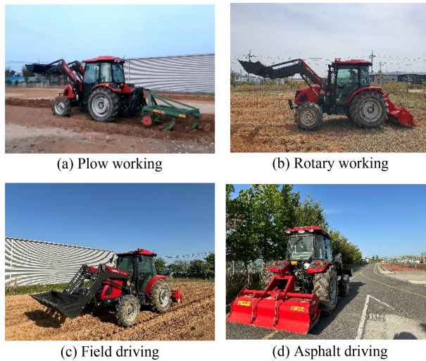
Fig. 5 Filed tests for an agricultural tractor
