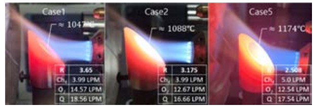
Fig. 10 Photos of flame for the three different burner rig test conditions
