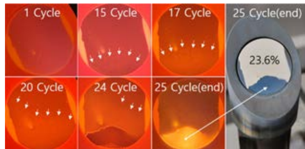
Fig. 16 The progress of specimen failure according to the number of cycles (Case3), photos taken at the second half of heating step, except for the farthest right
