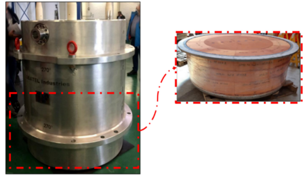
Fig. 9 Fenosol foam used to R-83 cask [29] (Adapted from Ref. 29 with permission)
